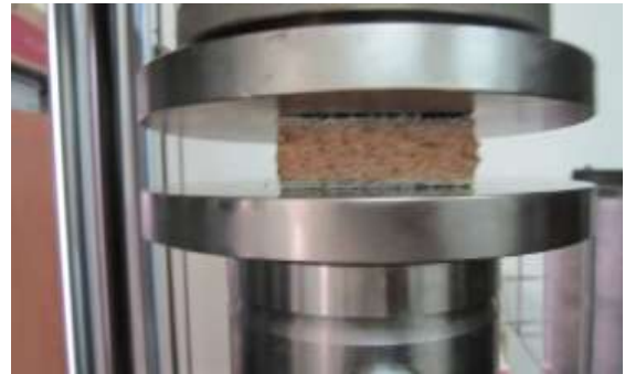
Figure 2. Specimen sandwich in the compression test.
