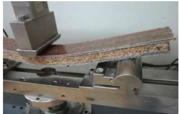
Figure 8. Bending tests three items, after fracture.
